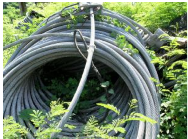
New strands was found in pretty poor condition
