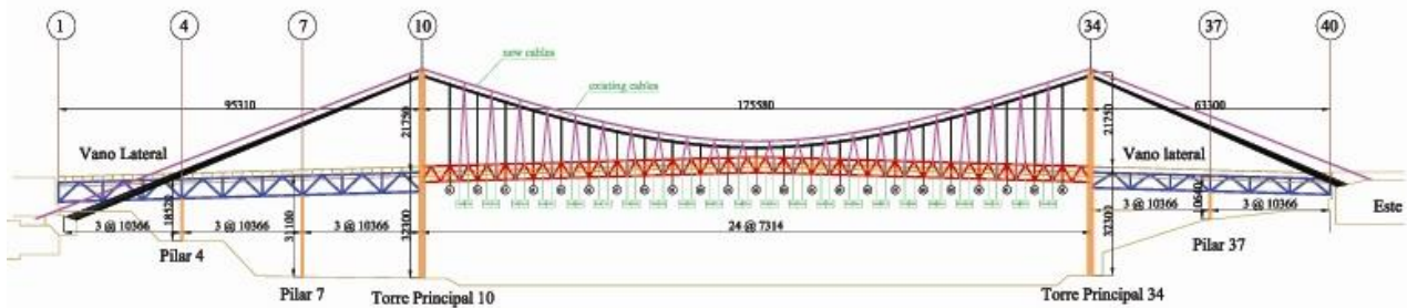
Puente Duarte elevation after reconstruction
